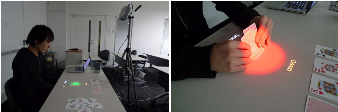
FIGURE 5.4: EmoPoker system and visual feedback example. The player's hand cards are spotlighted by the projector and the color indicates arousal level (e.g., blue: calm, red: aroused). RFID tags are attached to each card in an unobtrusive way so that poker game events can be implicitly tracked and recorded by the system.
